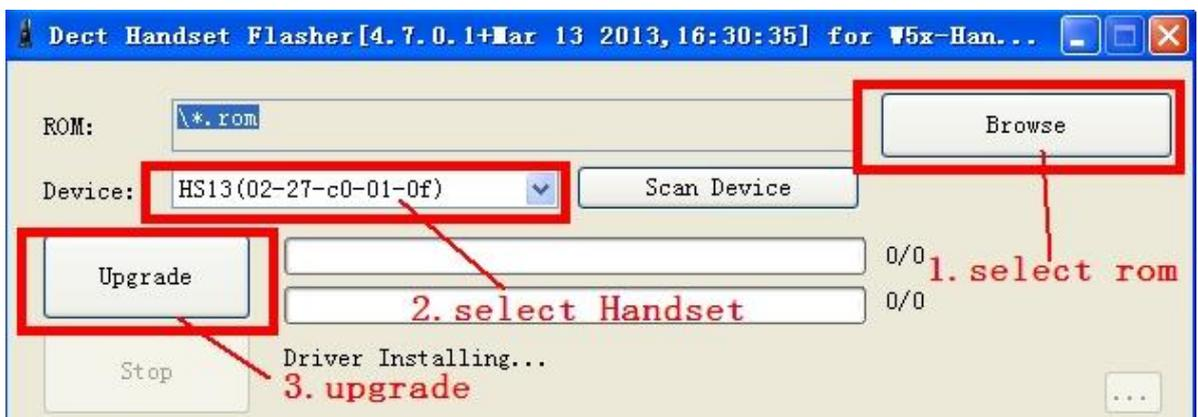
The tool will know the handset identification code (02-27-c0-01-0f) automatically, normally, it's begin at 0227cxxxx, if not, it may take mistake. The HS13 indicate COM port, you can find it through device manager.
